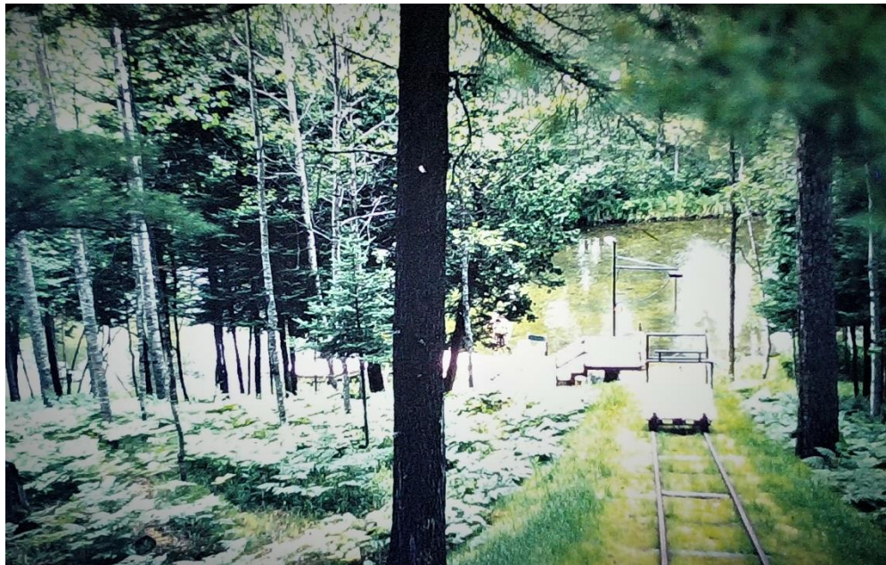
View of the elevator. Notice the chain falls on the dock at the end of the rail. These were used to off load the AuSable River Boat that we owned into or out of the river. The little “railing” at the back of the car was installed so the river boat could be level when transported down to the river. The device was powered by a 2 ½ horsepower overhead door motor and equipped with
